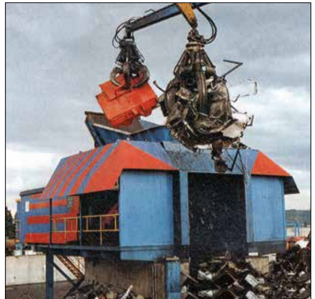
1992 S. PIERRE DE CAUDIEU. The first pre-shredder, with independent counter-rotating shafts.
