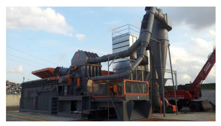
The "REDMILL" module, a horizontal axis hammers mill with side loading system, has been designed and built to enhance, through grinding and selection, the "poor" scrap from E.L.V, light scrap, WEEE, large home appliances ...
