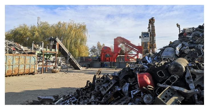
The "REDFINER" module enhances, through comminution and selection, the "poor" scrap coming from separate collection, WEEE, small appliances, valves, casings, internal combustion engines from end-of-life vehicles, cans, spray cans, electric motors, transformers, stators, window frames, packaging scraps, meatballs......
