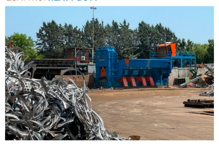
The purpose of the shear balers is simple: to cut and densify scrap to optimize storage space, reduce transport costs and supply the scrap "ready to furnace".
