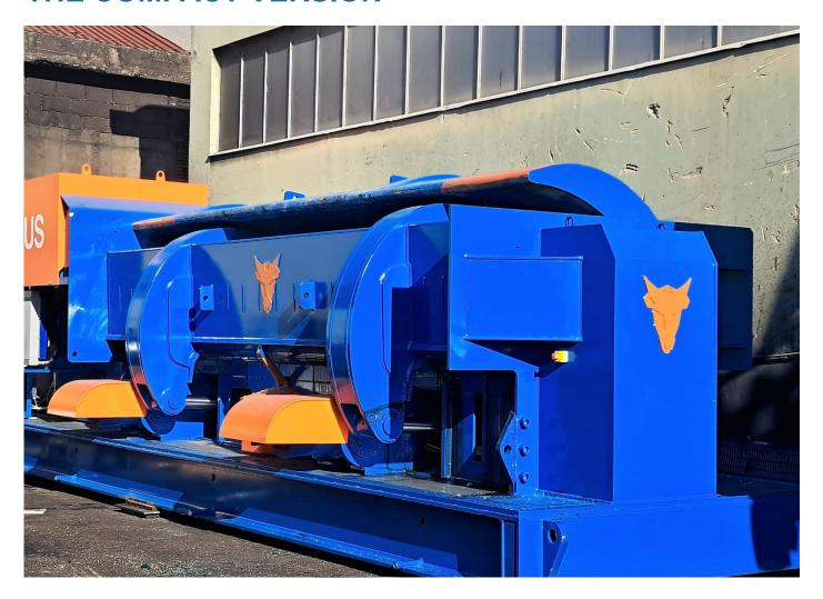
The new "KEF" baler line consists of a single monolithic structure, does not require foundations and is easy to install and reposition.
