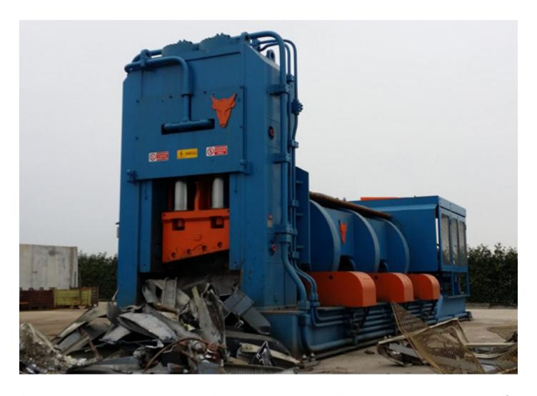
The scrap industry is undergoing a radical change, to which dedicated technologies must adapt. So no more foundations, ancillary structures and bureaucratic headaches. The shear baler can enter the scrap yard without disturbing production, be placed on the floor and operate within a few days of delivery. When its useful life is over, it can be dismantled quickly.
