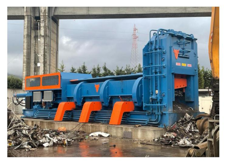
The COMPACT shear baler is a versatile machine, suitable for processing different types of scrap. The COMPACT shear baler has a single monolithic body on a self-supporting frame, requiring no foundations and no special permits.
