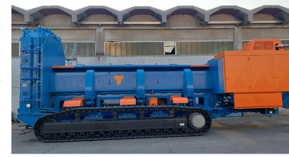
The shear baler "CAT" series are made up of a single self-supporting monolithic structure. The "CAT" shear is equipped with the original TAURUS SB compression box with over-stroke on both wings.
