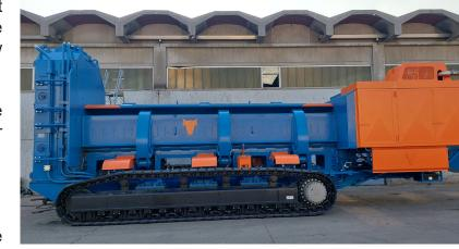
The shear baler "CAT" series are made up of a single self-supporting monolithic structure. The "CAT" shear is equipped with the original TAURUS SBxc compression box with over-stroke on both wings.
