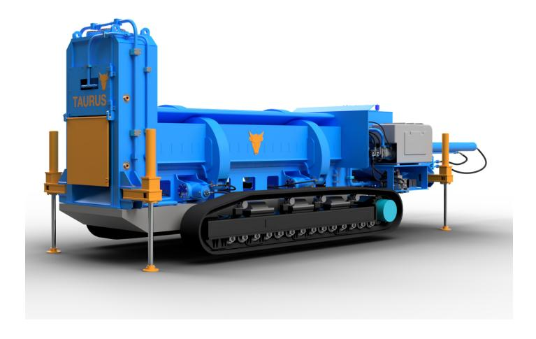
CATJ transportable shears balers are equipped with 4 lifting cylinders to ensure ground alignment. Furthermore, the cylinders allow the lifting of the shear permitting the loading and unloading on the means of transport, whether it is a tracked vehicle or a swan neck trailer.
