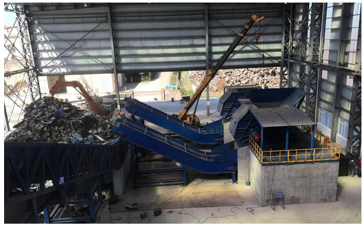
The BRAVO 'redripper', with horizontally counter-rotating shafts, is used upstream of hammer mills in scrap mills, to coarsely and homogeneously crush mixed scrap, bulky scrap and E.L.V. It is in particular used to rip bales of E.L.V., light and collected scrap, to facilitate feeding and make uniform the subsequent ripping operation at the mill.
