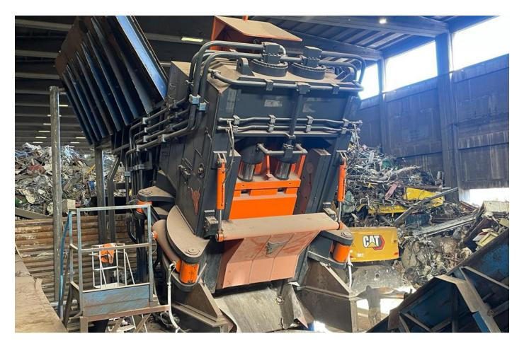
The BLACKLINE TR inclined shears, have been revised, updated and completed. The range has been extended with the introduction of TR-VHD (very heavy duty) shears with cutting forces of up to 1,800 tons, suitable for continuous shearing of any type of scrap, from profile, pipes, steel sheets to mixed and bulky scrap, demolition, rails, rebar, bales, etc...
